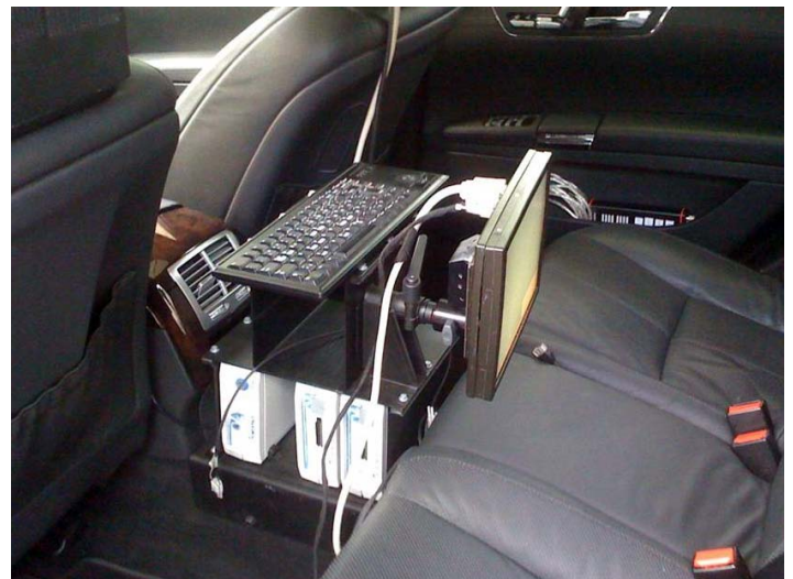
Online analysis and monitoring of driver's vigilance, BrainVision RecView modules programmed by Daimler
