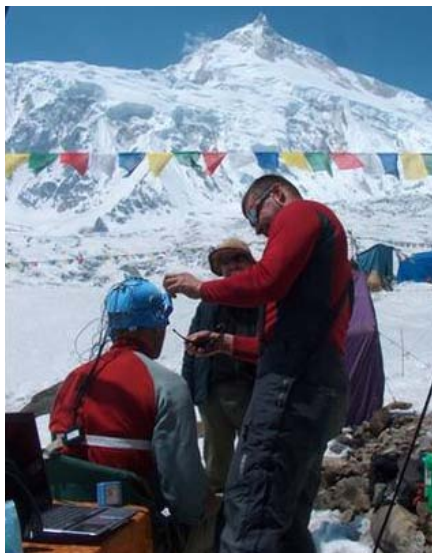
Pic. 1: EEG cap preparation at 4.800 m: a member of the expedition fills the electrodes in with SuperVisc gel
