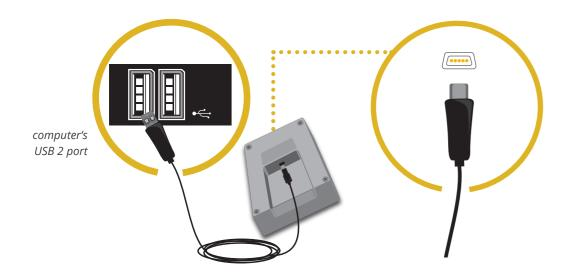
Remove the battery cover on the rear side of the ControlBox. Then use the actiCAP USB cable to connect the ControlBox to the computer. Windows will install the driver automatically.
