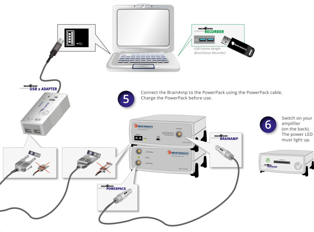
After use: Disconnect the PowerPack from the amplifier and immediately recharge the PowerPack.
