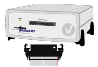
Installing the dongle: Plug in the USB dongle. The dongle driver is installed automatically. When installation is complete, the dongle will light up.
