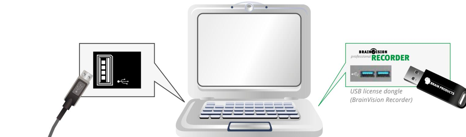
**3** **Installing the USB2 Adapter:** Use the USB cable to connect the USB2 Adapter to your computer. Windows will detect the new hardware and install it automatically.
