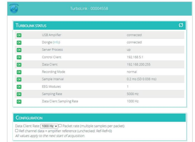
Example: Recorder sampling rate is 5000 Hz. If "Data Client Transfer Rate" is 1000 Hz and "Packeting" is unchecked, the signal is down sampled to 1000 Hz. If "Data Client Transfer Rate" is 1000 Hz and "Packeting" is checked, packets of 5 samples are sent at a 1000 Hz rate.
