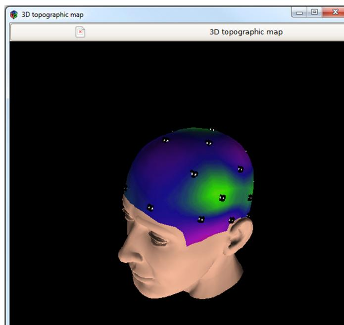
Fig. 2: The signals acquired by the actiCHamp can be visualized in realtime and in 3D with OpenViBE. This picture shows the beta-band power for 32 channels of the actiCHamp
